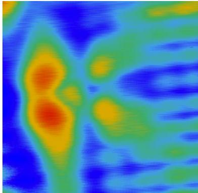
Figure 1: STM image (3nm x 3nm, -1.5V, T=4K) of a single Cr atom incorporated by the STM tip in a Ga position on the first plane of the GaAs(110) surface.
